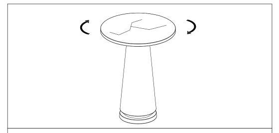
**STEP 3:** Gently rotate the top in a clockwise direction until firmly screwed in. \*Note-Tightening too much can damage the base insert.
