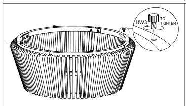
**STEP 4:** Place the base ring upside down and carefully tighten the levelers as shown above.
