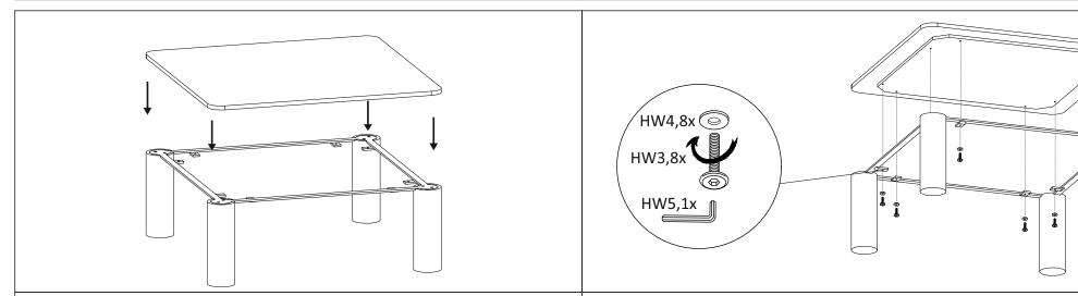
**STEP 3:** Place Marble Top carefully on the frame and align top with legs. **Note:-** Mind the fingers while placing the top over the metal frame.
