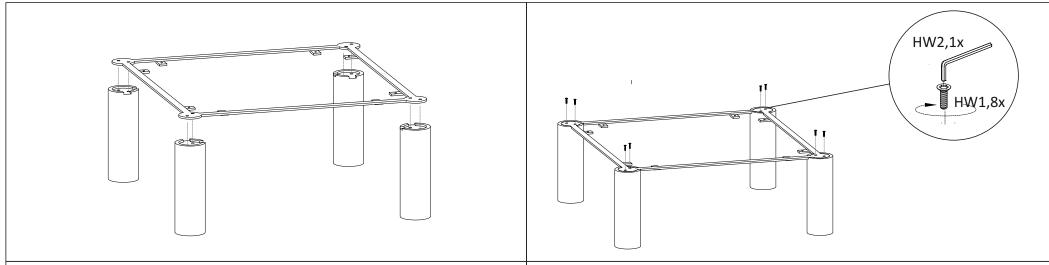
**STEP 1:** Place legs upright on a flat surface. Carefully align the metal frame over the screw holes in the legs.
