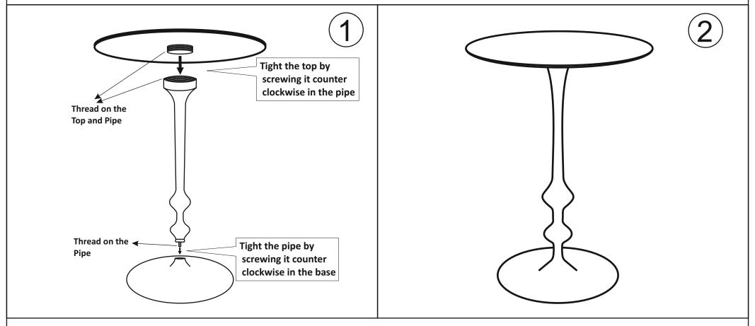
STEP 1 : TIGHT THE TOP BY SCREWING IT COUNTER CLOCKWISE IN THE PIPE AND TIGHT THE PIPE SCREWING IT COUNTER CLOCKWISE IN THE BASE
