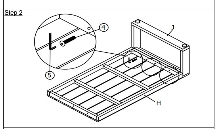
Place the Table Top(H) on a clean, non-marring surface. Then attach the Left Leg Panel(J) to the Table Top(H) by using Bolt(4) and Allen Wrench(5) as shown above.
