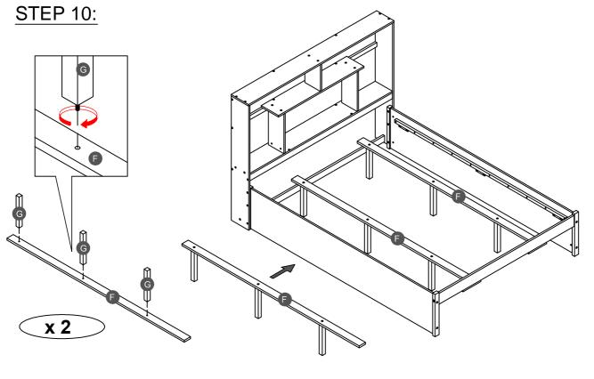
Assembling leg support (G) with lower support slat (F) later rotate, Move support slat inside Queen bed.
