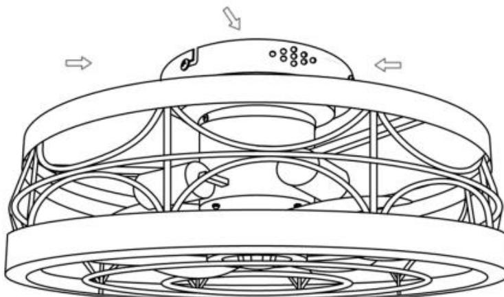
Place the two key holes from the ceiling fan over the two screws previously loosened from the hanging bracket. Turn the ceiling fan until it locks in place at the end of the key holes. Secure by tightening the two screws previously loosened and the one screw previously removed.
