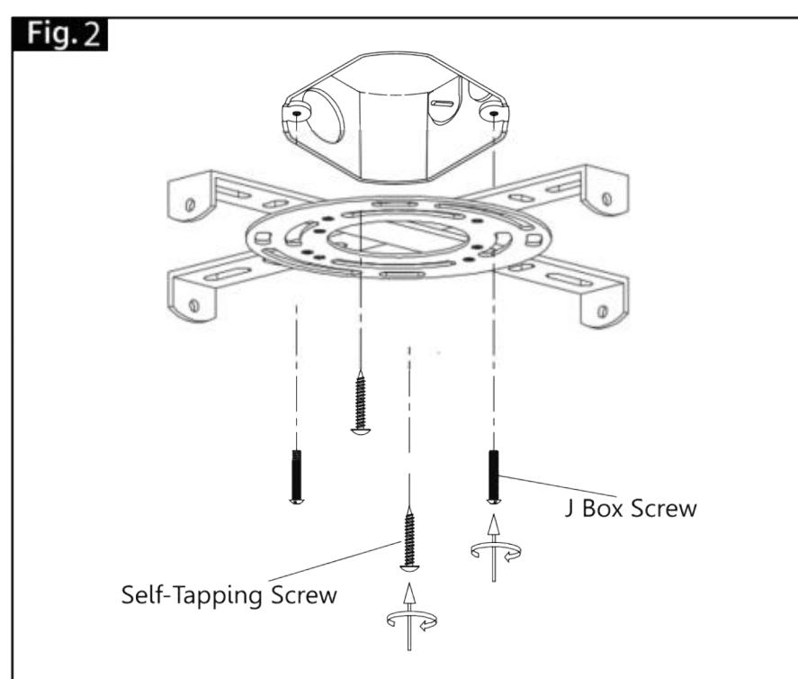
Attach the hanging bracket to the outlet box (not included) with the two J box screws provided. Secure the hanging bracket to the ceiling with the two self-tapping screws provided.
