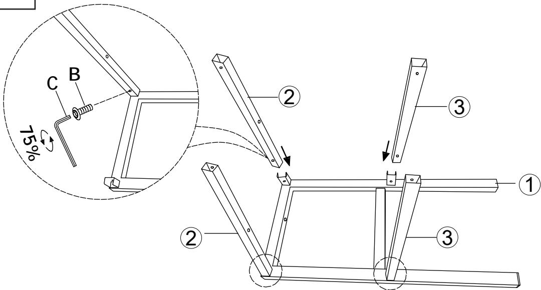
Remark: The difference between ② and ③ is that ② have holes at the bottom, which are used to install the seat in step ③. 75% means do not tighten completely.
