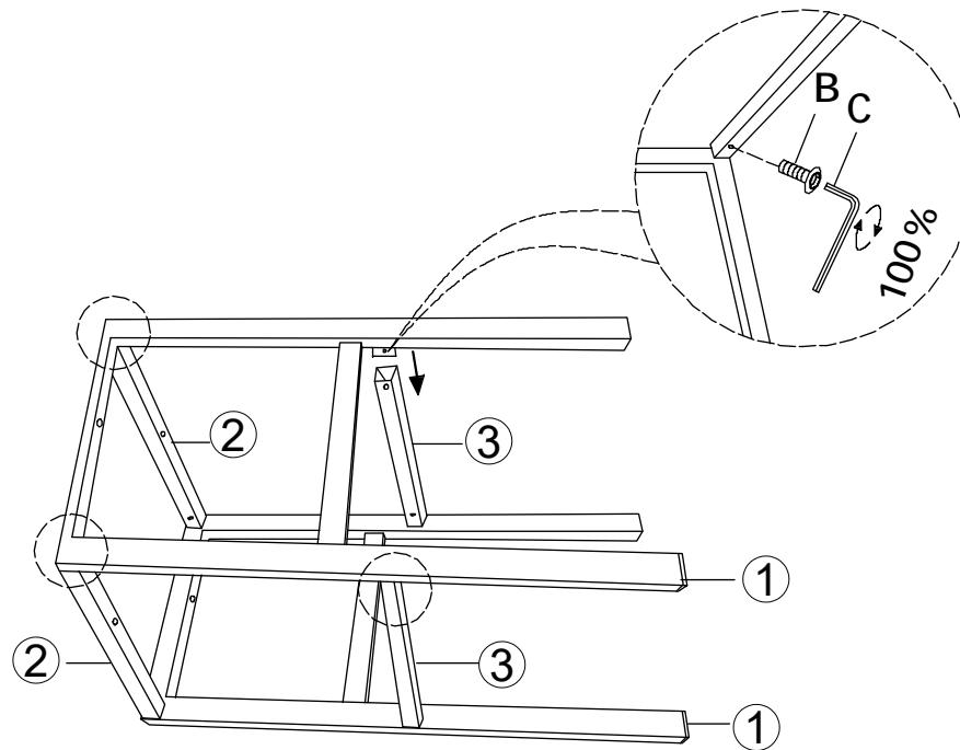
Remark: After installing the other leg ①, tighten all bolts in steps 1 and 2 to 100%.
