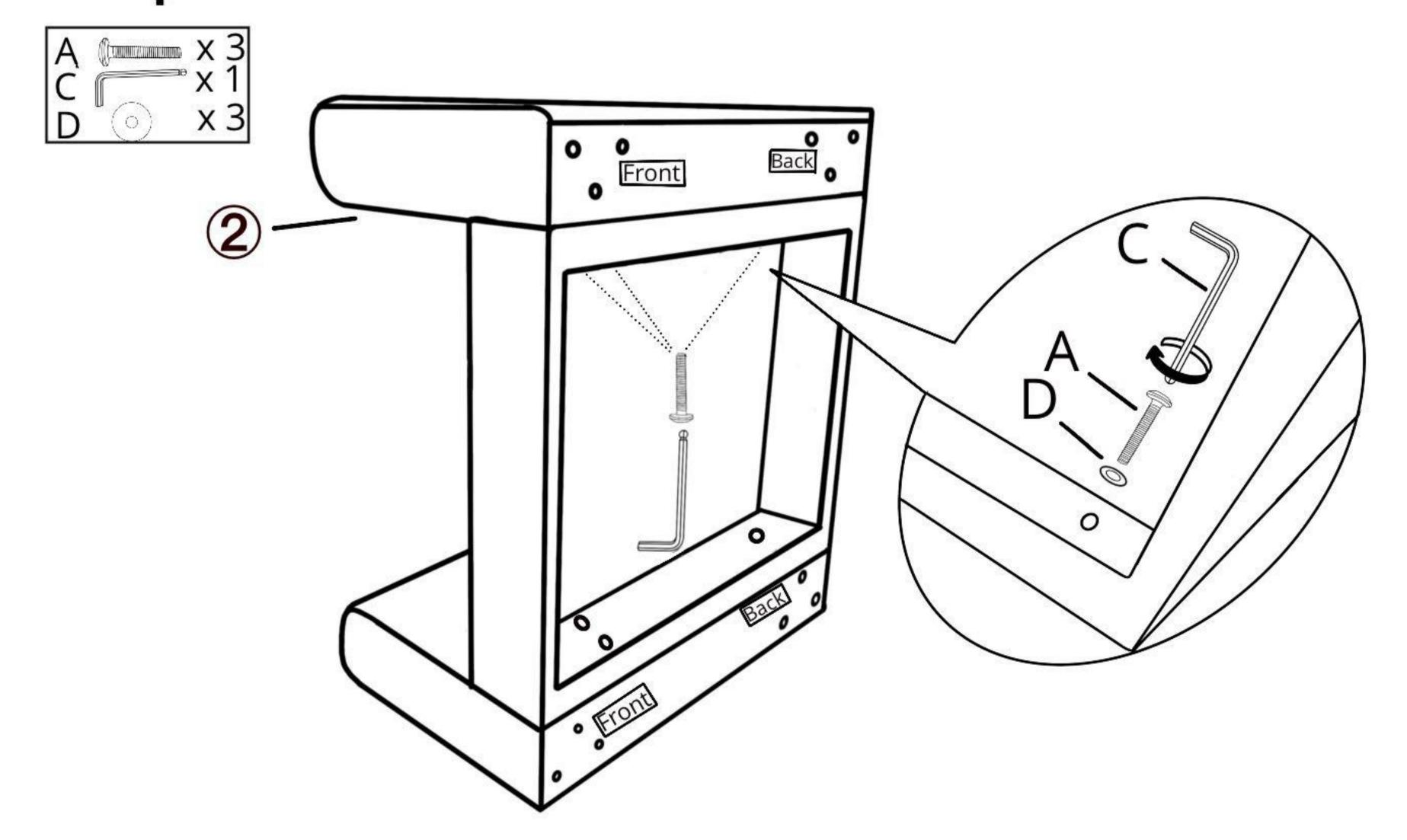
Kindly Remind: Please fully tighten the screws after all 3 screws are installed.
