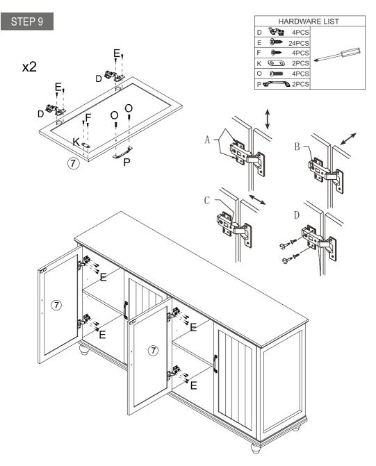
B.Depth adjustment D.After adjustment A/B/C,tighten screws.
