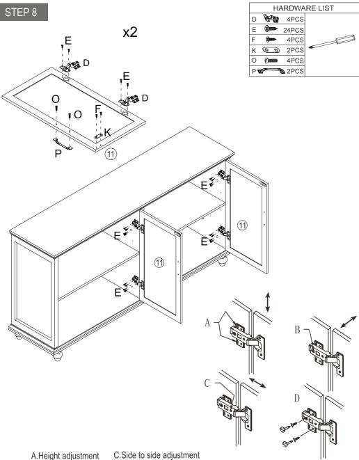
B.Depth adjustment D.After adjustment A/B/C, tighten screws.
