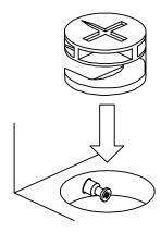
Turn the cam lock clockwise to tighten.
