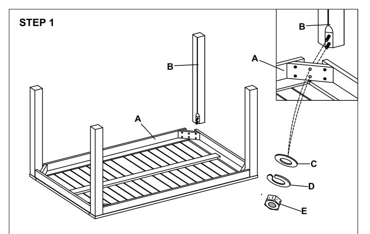
Attach the leg frames (B) into each corner of the table top (A). Assemble the washers (C), spring washers (D) and nuts (E) to leg frames (B). Tighten the nuts using wrench.
