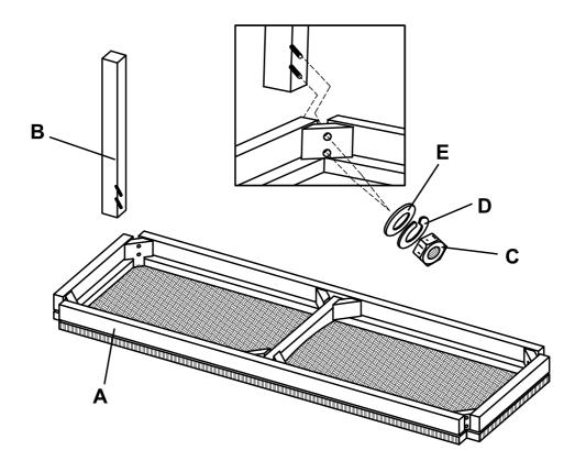
Attach the legs (B) into each corner of the Seat (A). Insert Washer (E), Spring washer (D), and Nut (C) to each legs (B). Tighten nuts using wrench.
