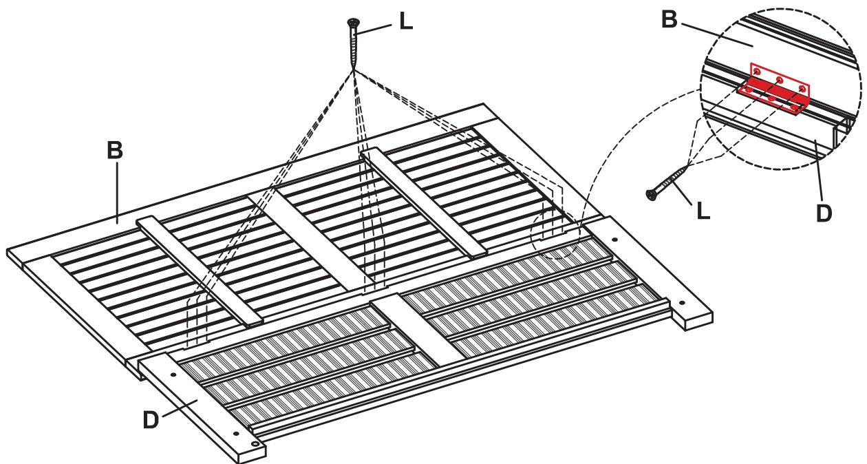
Attach the Top frame (B) to the back frame (D) on clean flat surface, secure with 5/8" screws (L) using screwdriver, position as shown.
