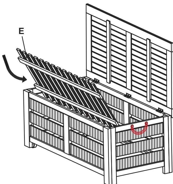
Put the slatted base (E) to the assembly from step 5, as shown. Tighten all bolts using screwdriver,
