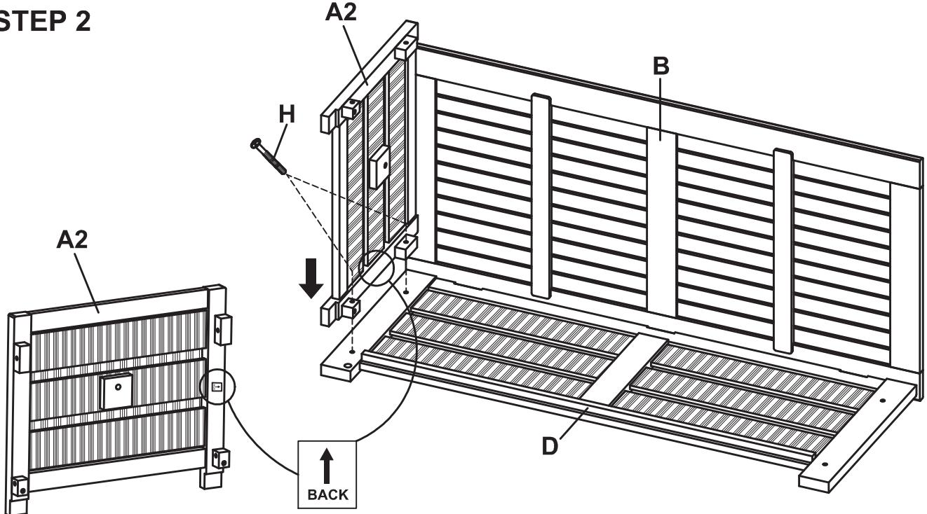
Attach the left side frame (A2) to the back frame (D). Secure with 1 1/2" Bolts (H) using screwdriver.
