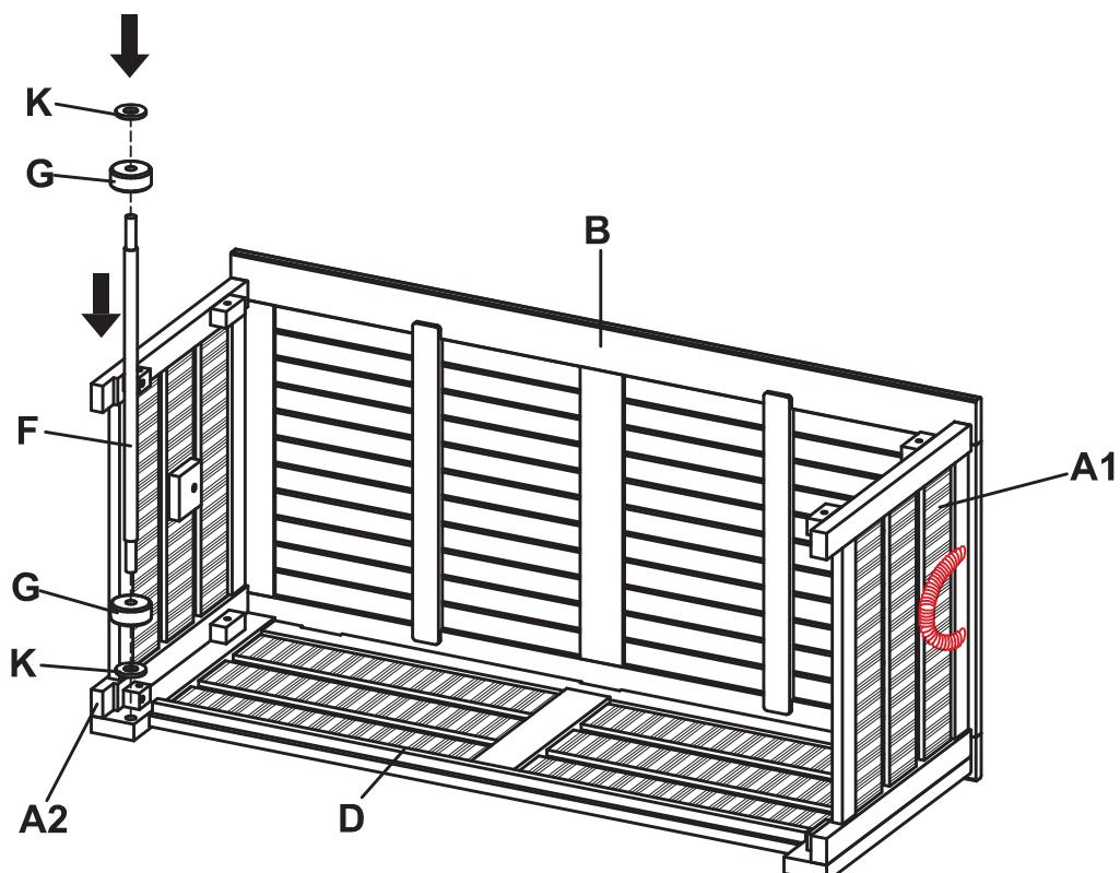
Attach Washer (K), wheel (G), and dowel (F) into back frame (D)
