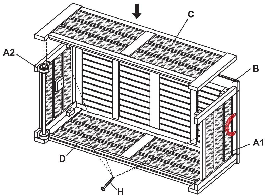
Attach front frame (C) to the right side frame (A1) left side frame (A2) and dowel (F). Secure with 1 1/2" bolts (H). **Do not fully tighten the bolts yet.**
