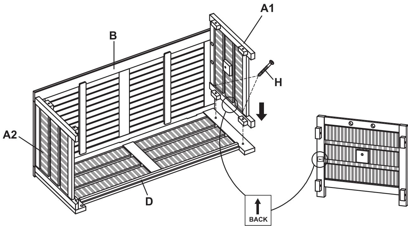
Attach the right side frame (A1) to the back frame (D). Secure with 1 1/2" Bolts (H) using screwdriver.
