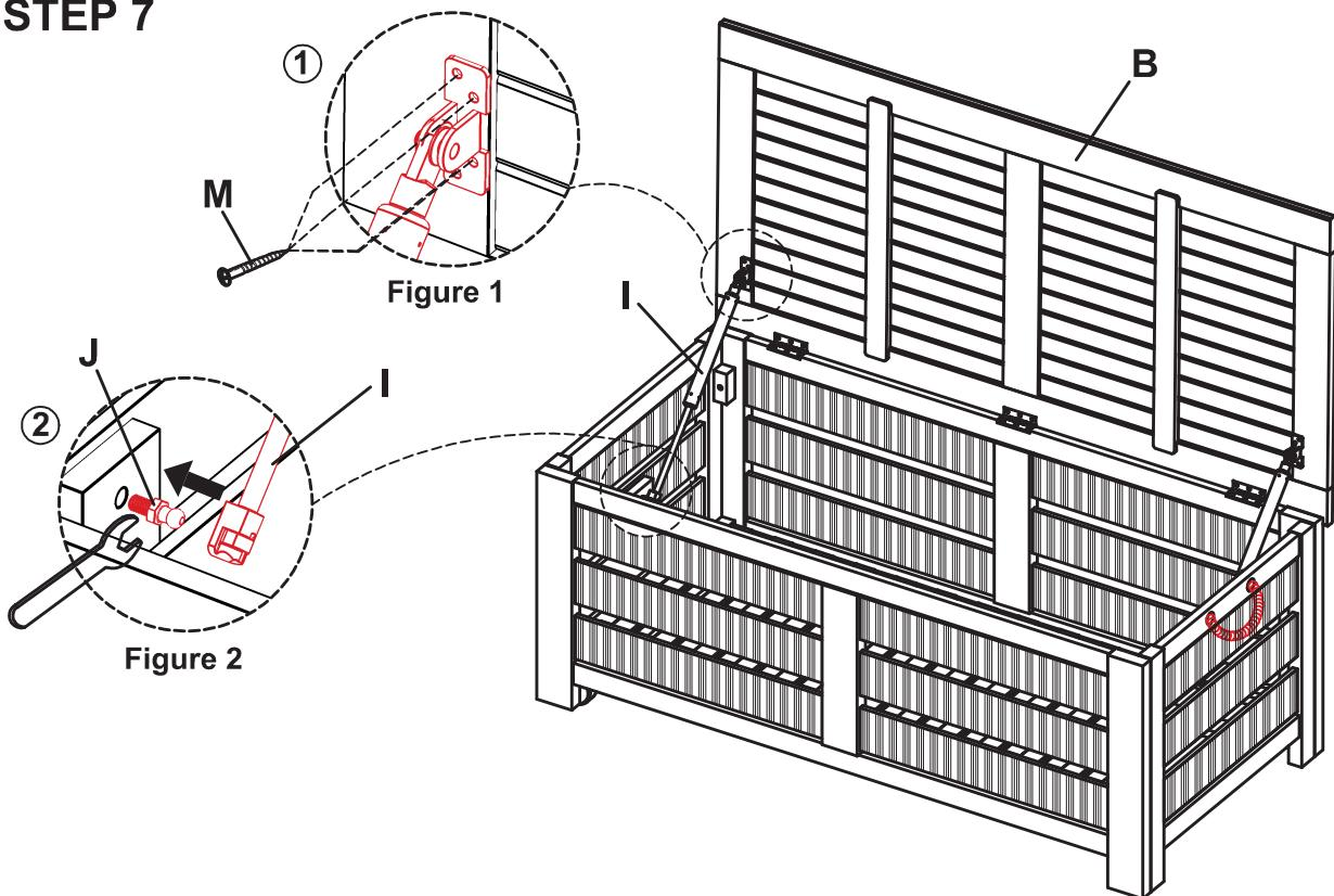
Attach lid support (I) into top frame (B), secure with 16 mm screws (M), as shown (figure 1).
