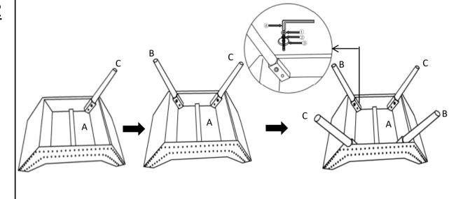
Install the legs on the leg position located on the underside of the Ottoman.
