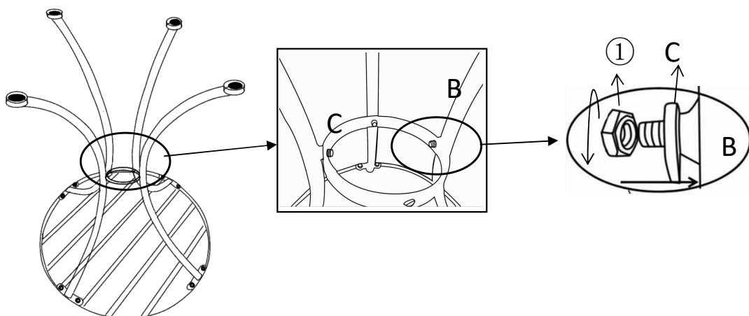
Attach the Support Ring(C) to Table Legs(B) using Nuts(①) with Spanner(②).
