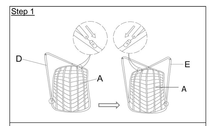
Open the carton and place all the parts onto a clean, non-marring surface. Please insert the Left Back Leg (D) into the Seat (A), then insert the Right Back Leg (E) into the Seat (A) as shown in the picture.
