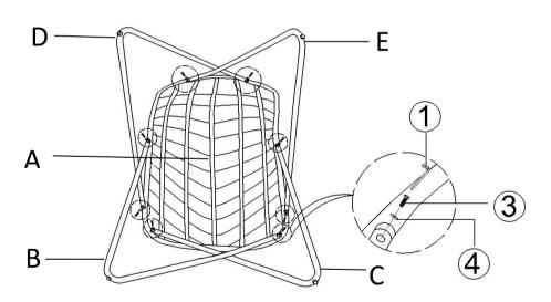
Attach the Left Back Leg (D), the Right Back Leg (E), the Left Front Leg (B) and the Right Front Leg (C) to the Seat (A) respectively, using Bolts (③) and Washers (④) with the Allen Wrench (①) as shown in the picture.
