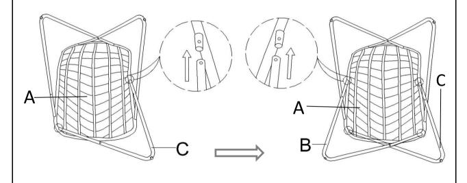
In the same way, insert the Right Front Leg (C) into the Seat (A), then insert the Left Front Leg (B) into the Seat (A) as shown in the picture.
