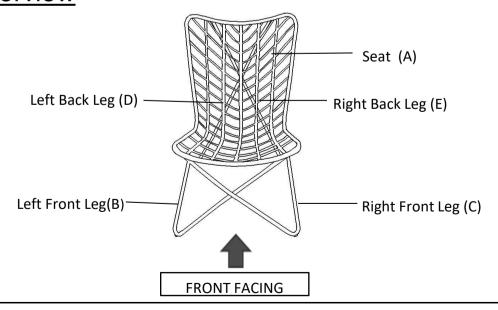
This Chair has multiple parts and may require up to some 30 minutes to assemble. To give you an overview of the Chair parts, the above picture is to help you put the various parts into perspective. Please read through the instructions below to familiarise yourself with the parts and steps before assembly.
