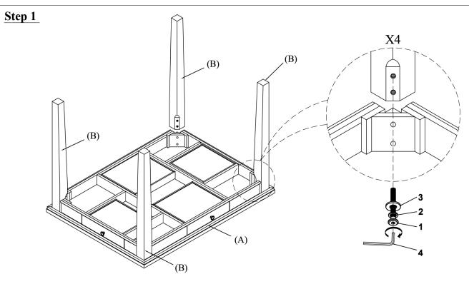
DO NOT TIGHTEN BOLTS UNTIL COMPLETELY ASSEMBLED.
