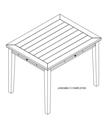
DO NOT TIGHTEN BOLTS UNTIL COMPLETELY ASSEMBLED.
