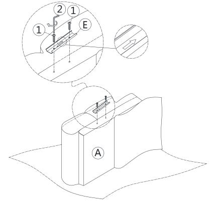
Be sure the blot  $\ (1)$  goes through the correct hole in the metal brackets  $\ (E).$
