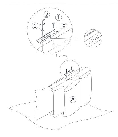
Be sure the blot (1) goes through the correct hole in the metal brackets (E).
