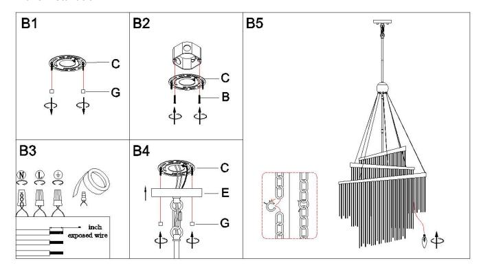
Step B1 » Unscrew ball nuts (G) from mounting plate (C).
