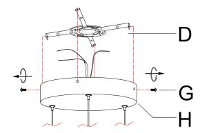
4 » Carefully pass the supply wires from the outlet box through mounting plate (D).
