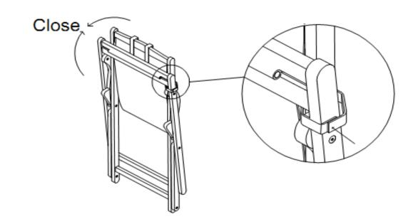
**Note:** There is a velcro straps beside Leg Frame, tie the velcro straps to Leg Panel as picture shown.
