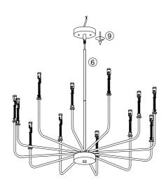
5.Let the wire go through the canopy  $\@$  , rotate to install the canopy on the hanging tube  $\@$ 0.
