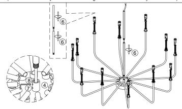
4.Let the wire go through the hanging tube ⑥, rotate to install the tube ⑥ on the connected tube ④,fix it with grub screw ⑦.
