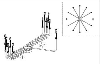
3.Adjust the arms  $\@3$  to suitable position like picture showed. (If the arm loosen, please back to step 2 to lock tighten with lock nuts  $\@3$ .)
