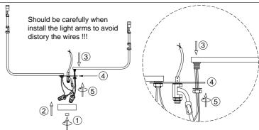
2.Fixed the light arms ③ to the fixture ④ with lock nuts & teeth lock washers ⑤, lock the bottom box ② to the fixture ④ with end cap ①.
