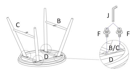
Align Center Cross Bar (E) to Left Leg (B) and Right Leg (C) then tighten Bolt with Lock Washer and Flat Washer (F) with Allen Wrench (J).
