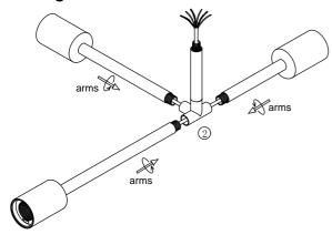
1.Rotate to fix the arms to the 4-ends connector ②.
