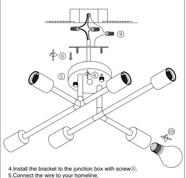
6.Install the light fixture to the bracket with cap nut<sup>®</sup>.
