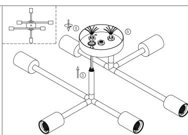
2.let the wire go through the canopy ⑤, lock the tube ③ to the canopy ⑤ with lock nut & teeth lock washer ④.
