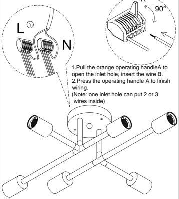
3.Connect all the wires by parallel with connectors ⑦(all live line-L use one connector, and neutral Line-N use another connector).
