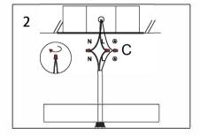
3. Install the canopy to the bracket with cap nuts D.
