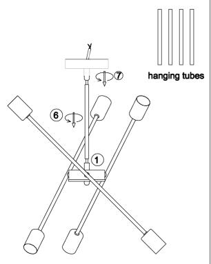
5.Let the main wire go through the hanging tube 6, turn to install the tube 6 on the fixture, after that let the wire go through the canopy 7, install the canopy 7 to the tube 6.
