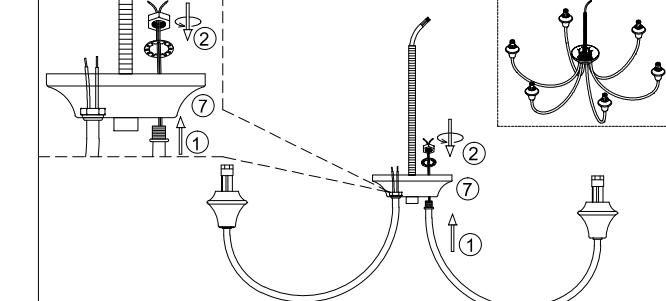
2. Install the light arms ① to the bottom ⑦ with lock nut & teeth lock washer ②, adjust the light arms to suitable position.
