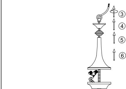
1. Rotate to remove out the hanging ring ③, bell shape cover ④, hanging ball ⑤, top cover ⑥.
