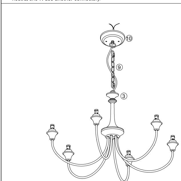
5. Hanging the light fixture to the canopy ⑩ with chain ⑨, let the wire go through chain ⑨ and the canopy ⑩.
