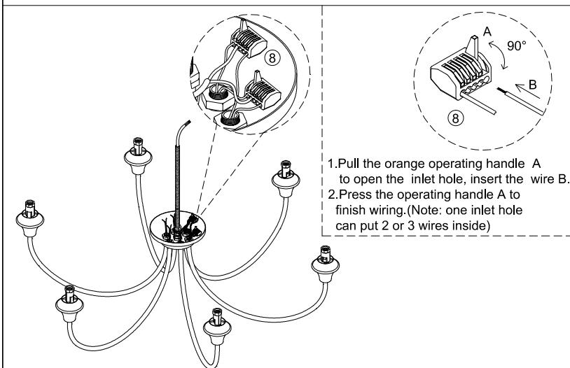
3. Connect all the wires by parallel with connectors ⑧ (all live line-L use one connector and neutral line-N use another connector).
