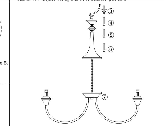
4. Let the main wire go through the top cover ⑥, hanging ball ⑤, bell shape cover ④ and hanging ring ③, rotate the ring ③ to make the parts fixed.
