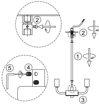
1. Let the wire go through the hanging tube ① and round plate set ②, rotate to install both to the fixture, fixed the tube ② to the fixture with grub screw ④ by rotate hex key ⑤, and fixed the round plate set to the tube with mini screw.
