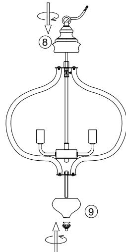
3. Let the wire go through the top cover group, rotate to install to the fixture, close the bottom cover with end cap ⑨.
