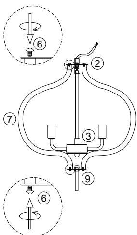
2. Install the metal profile ⑦ from hole of round plate ② to hole of bottom round plate ⑨ with bolt screw ⑥.
