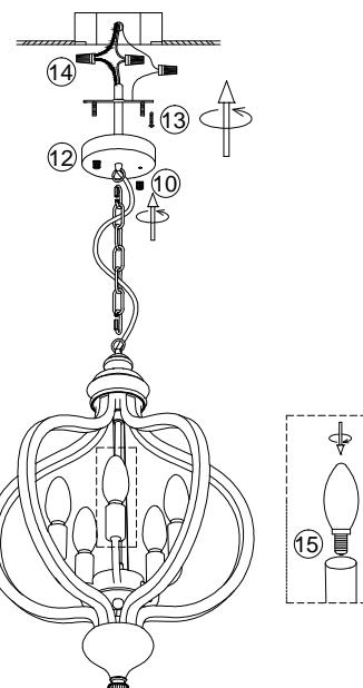
5. Install the bracket to the ceiling junction box with screw ⑬.
