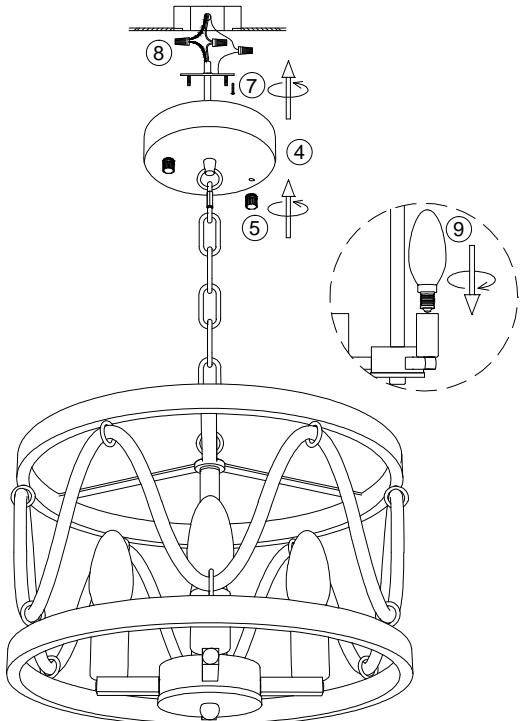
2. Let the wire go through the lampshade ③ and chain ⑥, rotate to fix both to the fixture ①.
