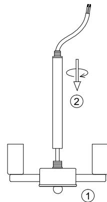
1. Let the wire go through the tube ②, rotate to install the tube ② to the fixture ①.
