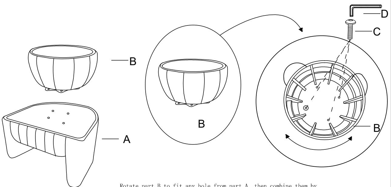
Rotate part B to fit any hole from part A, then combine them by tightening the screws to 80% firstly. Turn around part B to make every hole combined by tightening screws one by one to 80%. Then tighten all screws to 100% after all steps settled down.
