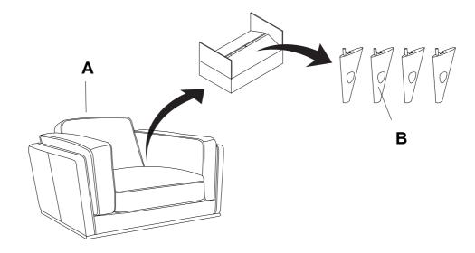
Put the Chair (A) on a smooth flat surface and attach Leg (B) to the Chair (A) using Bolt (C), Lock Washer (D) and Flat Washer (E) on the hole of Chair (A). Turn the Allen Wrench (F) in Bolt (C).
