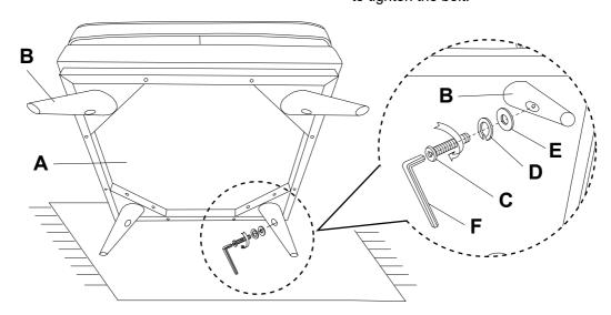
Stand chair up on an even surface and check that it is balanced. If there is a slight wobble, apply downward pressure in the corner where a leg is uneven. Keeping pressure in that corner, tighten all bolts. If balanced, apply downward pressure evenly in the center and tighten all bolts. Do not over-tighten beyond hole depth.
