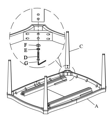
Turn the Table upright on a flat surface so that the Table will not wobble. Tighten all Allen Bolt (D) by using Allen Key (G). Unlock the sash locks underneath the Table Top (A).
