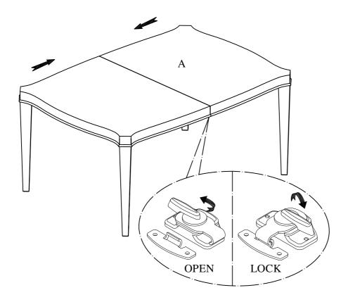
3 Pull out the Table Top (A) from both sides and put the Table Leaf (B) in the middle.
