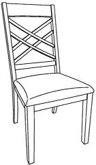
Helpful Tip: Instead of applying downward pressure while reaching under to tighten bolts, have someone sat on the chair while you tighten the bolts.
