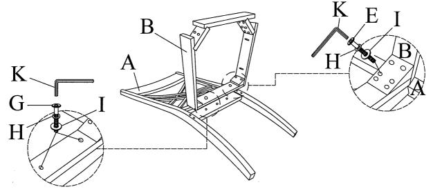
Take the Allen Wrench, and turn the bolts until the legs are secure. DO NOT TIGHTEN COMPLETELY.
