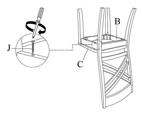
4 Stand chair up on an even surface and check that it is balanced. If there is a slight wobble, apply downward pressure in the corner where a leg is uneven. Keeping pressure in that corner, tighten all bolts. If balanced, apply downward pressure evenly in the center and tighten all bolts. Do not over-tighten beyond hole depth.
