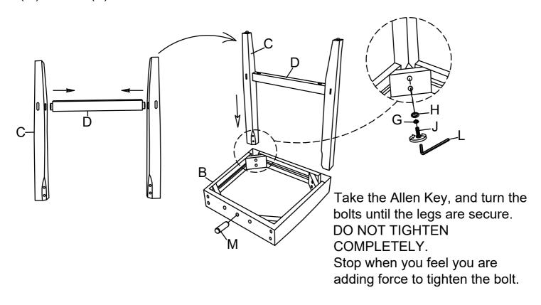
Put Chair Back (A) on a smooth flat surface, attach the Seat (B) to the Chair Back (A) using Bolt (I) & Bolt (K), Lock Washer (G), Flat Washer (H) in both holes of Seat (B) and Chair Back (A). Turn the Allen Key (L) in Bolt (I) & Bolt (K).
