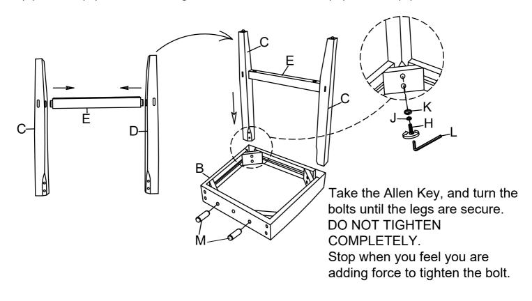
Put Chair Back (A) on a smooth flat surface, attach the Seat (B) to the Chair Back (A) using Bolt (G) & Bolt (I), Lock Washer (J), Flat Washer (K) in both holes of Seat (B) and Chair Back (A). Turn the Allen Key (L) in Bolt (G) & Bolt (I).
