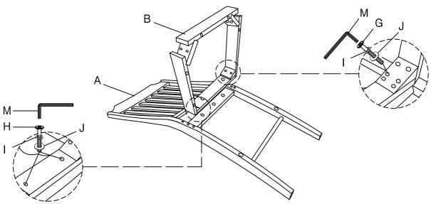
Take the Allen Wrench, and turn the bolts until the legs are secure. DO NOT TIGHTEN COMPLETELY.
