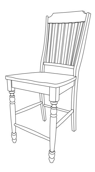
Stand chair up on an even surface and check that it is balanced. If there is a slight wobble, apply downward pressure in the corner where a leg is uneven. Keeping pressure in that corner, tighten all bolts. If balanced, apply downward pressure evenly in the center and tighten all bolts. Do not over-tighten beyond hole depth.
