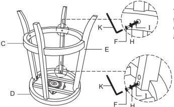
Take the Allen Wrench, and turn the bolts until the legs are secure. DO NOT TIGHTEN COMPLETELY. Stop when you feel you are adding force to tighten the bolt.
