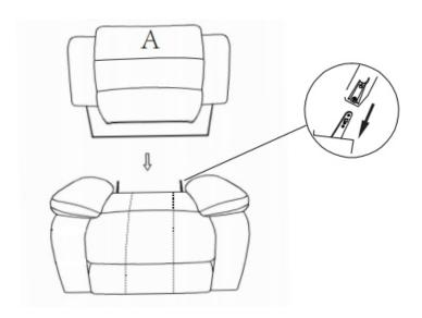
Uncover the back cover of the backrest, align the metal connector preinstalled on the inside of the backrest with the connector tip on the rear side of the seat, and press down vigorously to make the connector fully bite.
