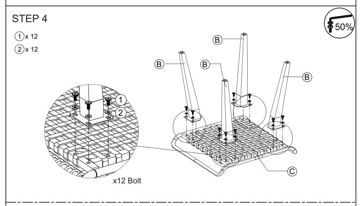
Connect the seat stool (C) & leg (B), tighten bolt (1), flat washer (2) with allen key (3).
