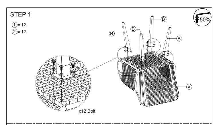
Connect the chair (A) & leg (B), tighten bolt (1), flat washer (2) with allen key (3).
