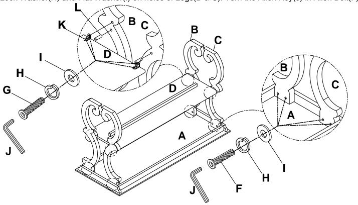
Attached Bottom(E) to the Legs(B & C). Use Allen Bolt(F), Lock Washer(H), Flat Washer(I) and Dowel(L) on holes of Bottom(E). Turn the Allen Key(J) in Allen Bolt(F).
