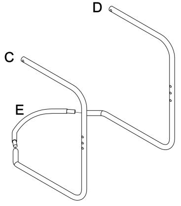
Step 3. Attach support legs (parts C & D) to chair back (part A) and chair seat (part B) using long bolts (part #1), round plastic washers (part #9), hex nuts (part #4), flat washers (part #5), plastic washers (part #8), wrench (part #6) and allen wrench (part #7).
