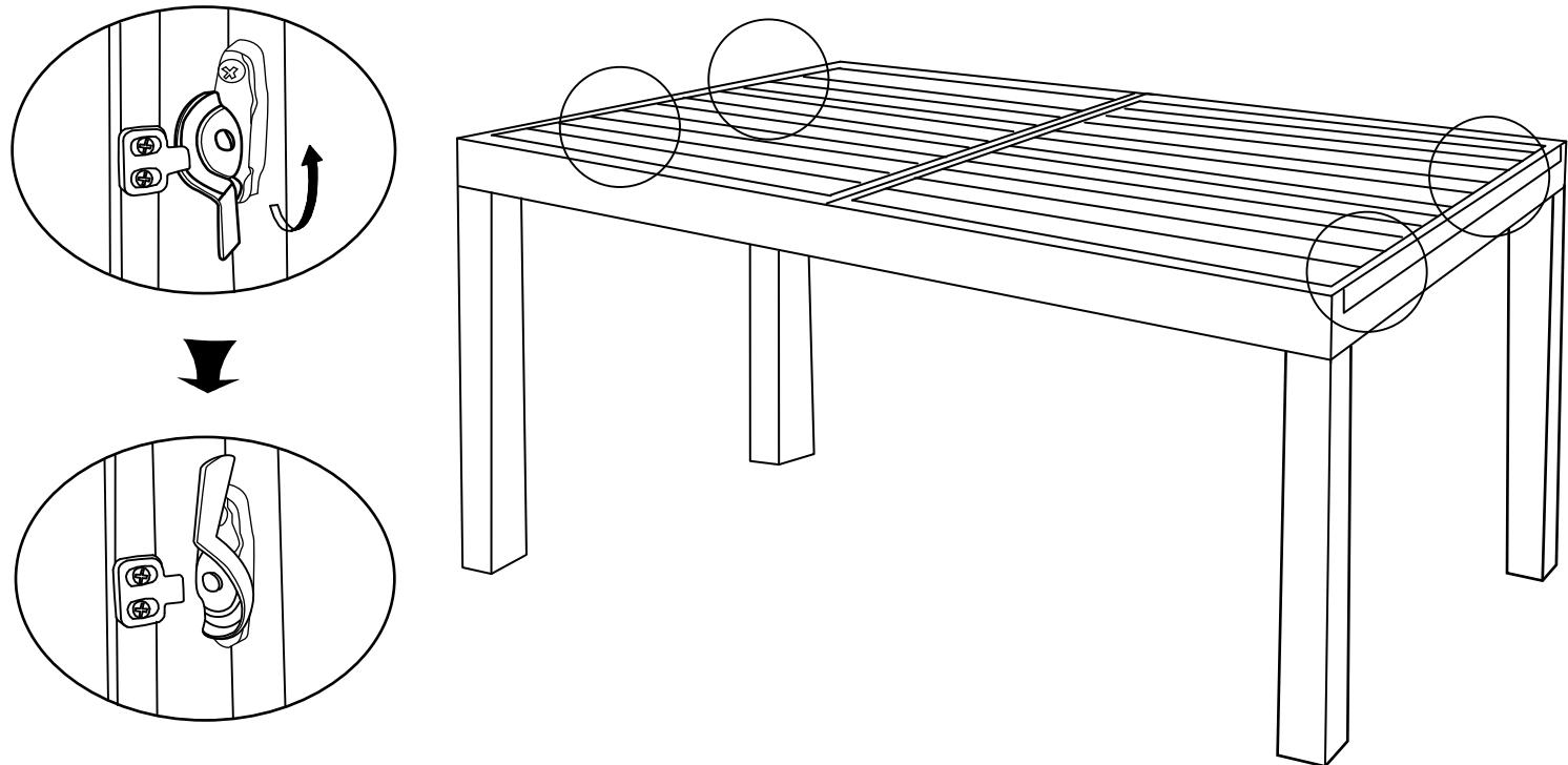
**B** Pull the left and right side panel outwards to extend the table.
