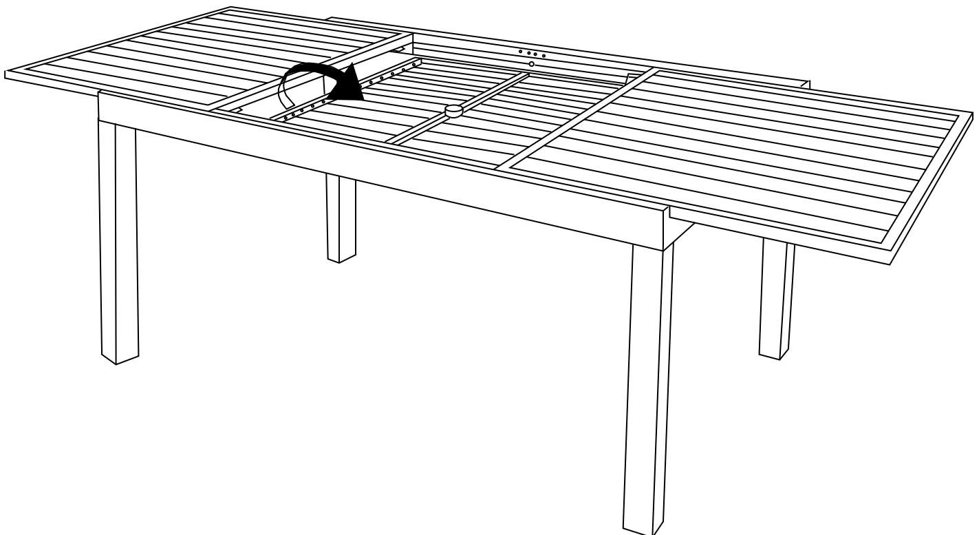
**D** Push the left and right panel to firmly close to the middle panel.
