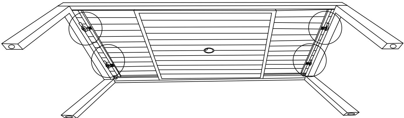
**B** Unscrew the side panels screws and nuts.
