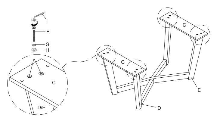
2 Lock Allen Bolt (F), Lock Washer (G), Flat Washer (H) on the holes of Leg (D & E) by Allen Key (I).
