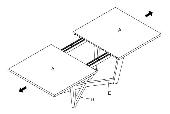
Attach Leaf (B) to the Table Top (A). Then push two sides of the Table Top (A) to reach the Leaf (B).
