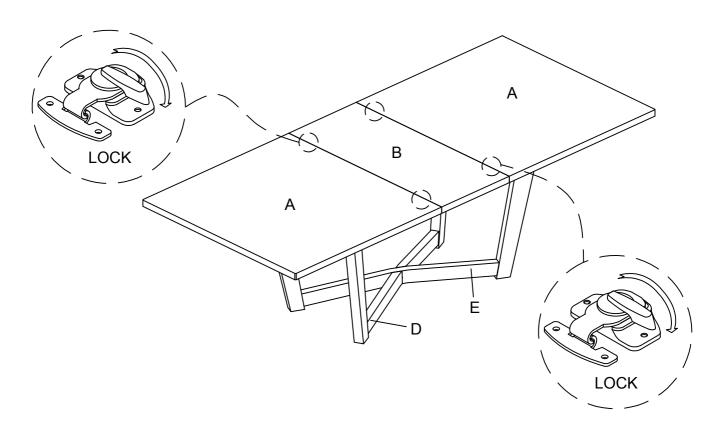
Adjust the Levelers at the bottom of Leg (D & E) to keep the table level.
