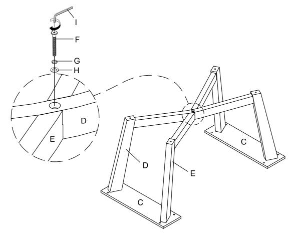
Attach Mounting Plate (C) to the Table Top (A) by Allen Bolt (F), Lock Washer (G), Flat Washer (H) and Allen Key (I).
