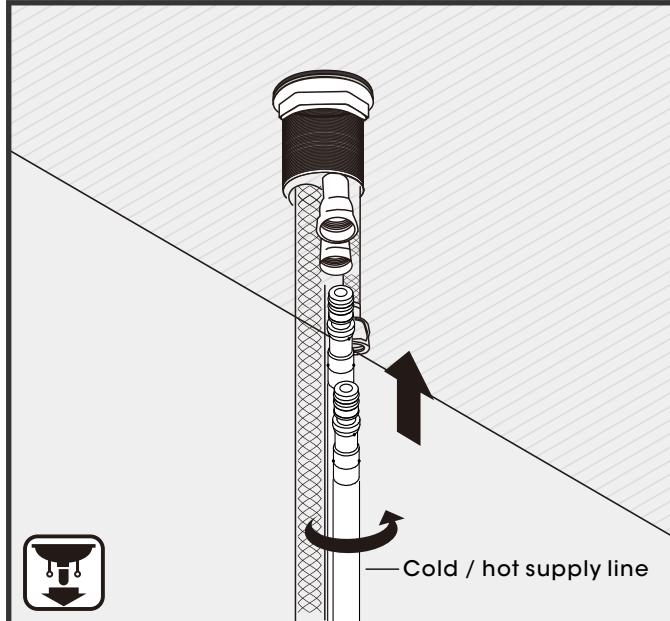
Connect the supply hose into the main water inlet hole.
