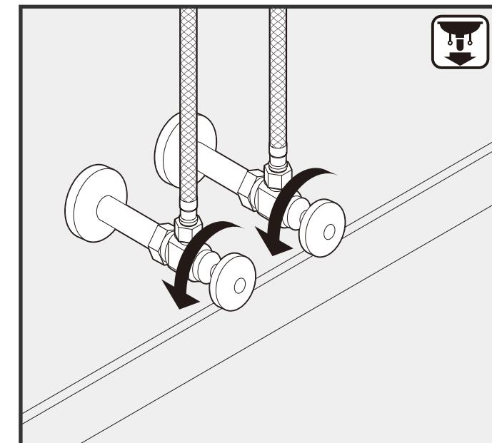
Turn the water supply line valves on and check for leaks.
