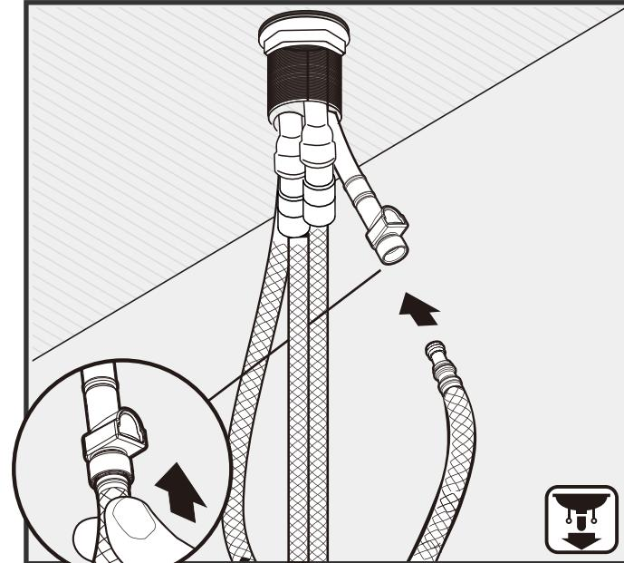
Push the quick connector firmly upward and attach it to the receiving block. Pull down moderately to ensure the connection has been made.
