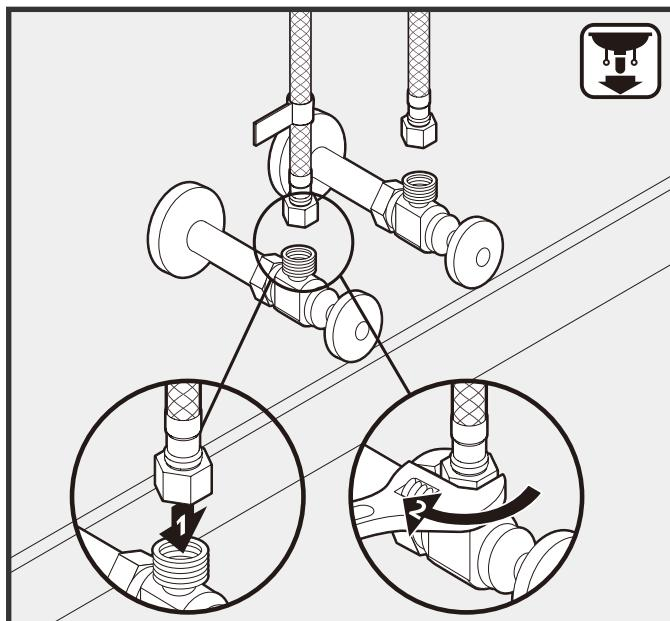
Attach flexible supply lines to shut off valves.Tighten with a wrench.
