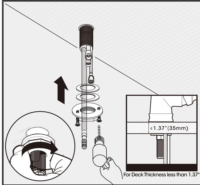
From underneath the sink, Push the faucet assembly up over the threads until it stops against the bottom of the sink, then hand turn (clockwise) to tighten.secure the faucet assembly to the sink .
