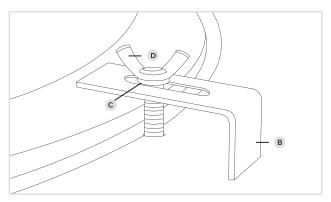
STEP 5 - ATTACH UNDERMOUNT CLIPS
