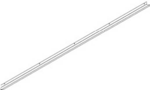
G02 GUTTER - A4M02570 (x2) 1 9/16"x1 15/16"x92 7/8" (40x50x2359)
