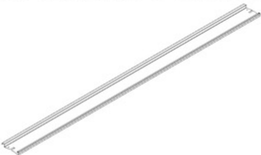
L01 LOUVER ASSEMBLY - A4M01995 (x28) 1 11/16"x7 3/4"x114 5/16" (42x196x2904)
