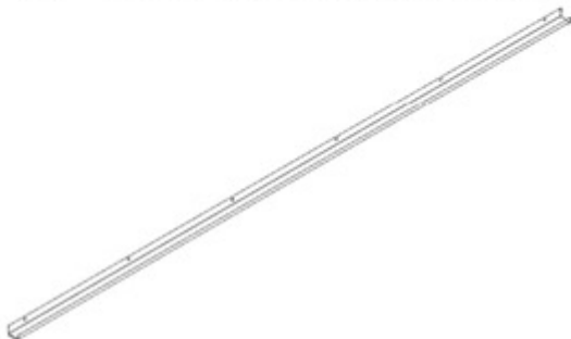
G01 GUTTER - A4M01993 (x2) 1 9/16"x1 15/16"x108 7/8" (40x50x2764)
