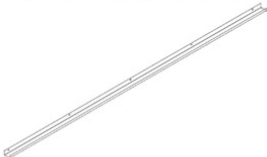
G03 GUTTER - A4M02571 (x2) 1 9/16"x1 15/16"x92 7/8" (40x50x2359)
