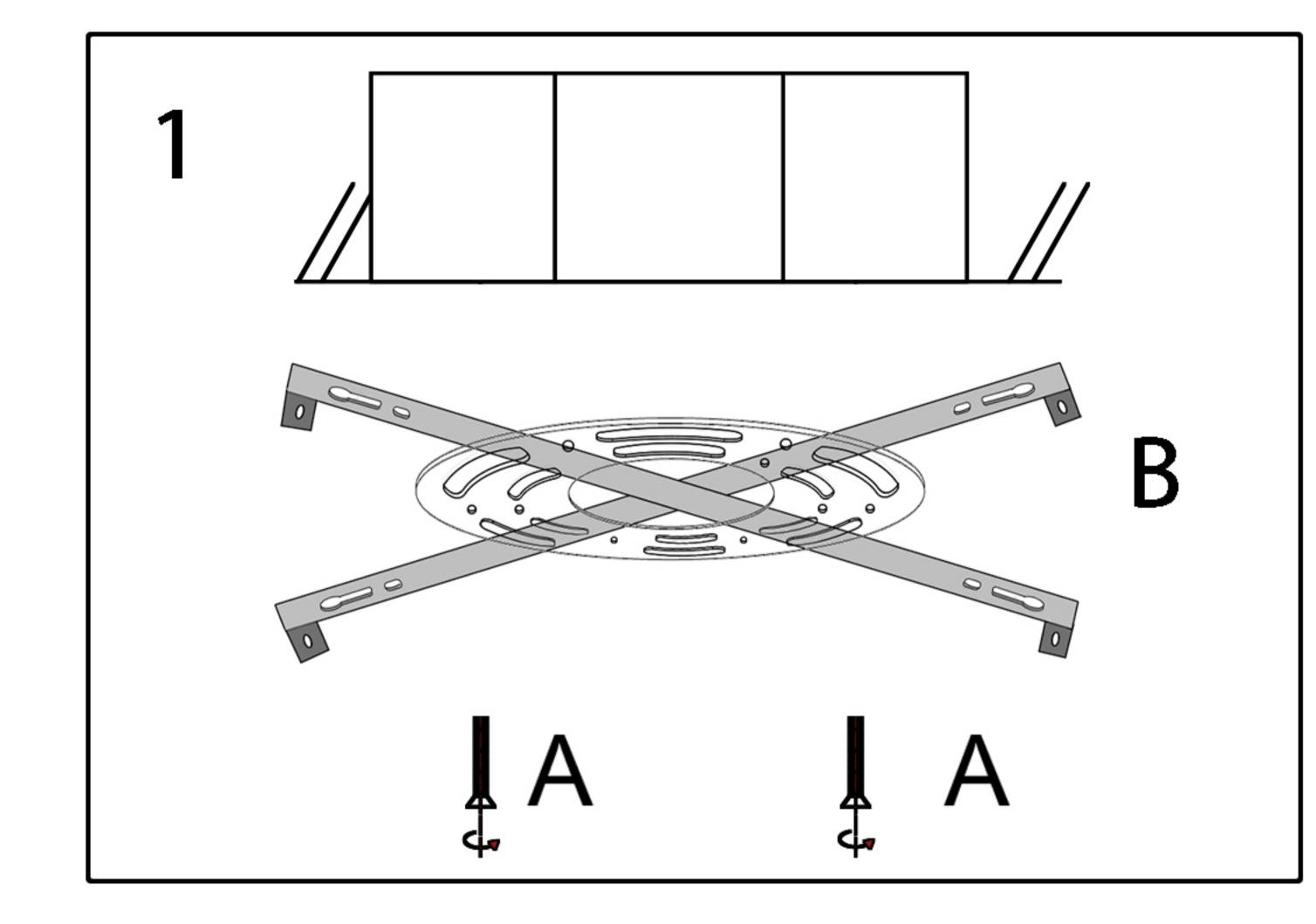
1.Install the bracket B to the ceiling junction box with screw A.
