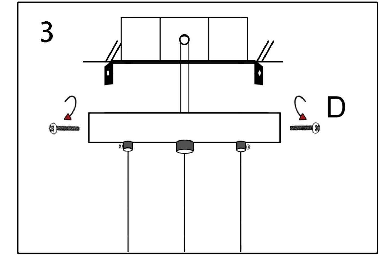
3. Install the canopy to the bracket with screws D.
