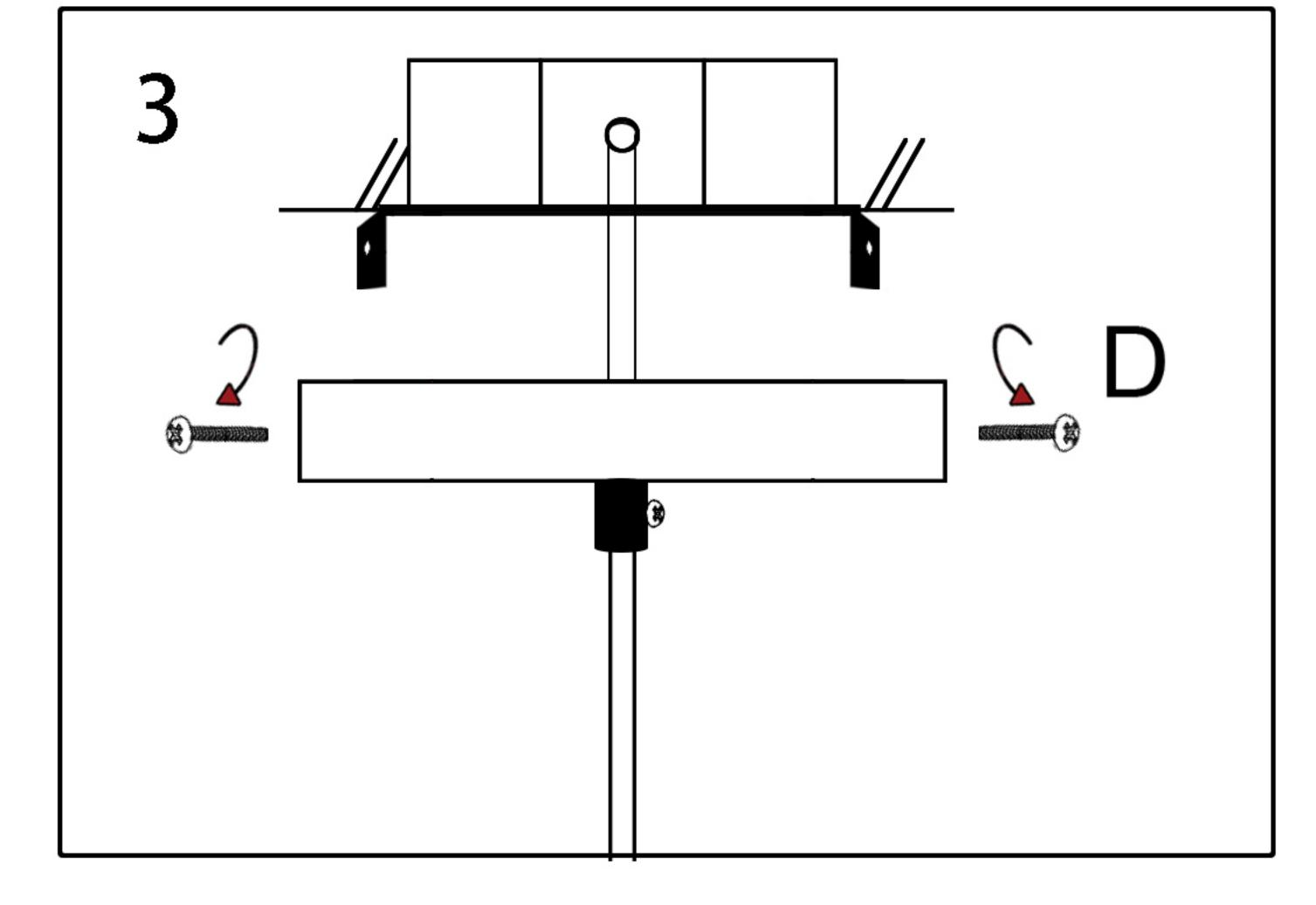
3. Install the canopy to the bracket with screws D.
