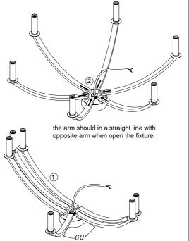
2.Let the wire of the fixture ① go through the big hanging tube ③, rotate to fix the tube ③ on the thread rod ②, let the wire go through the small tube ④, rotate the tube ④ on the big hanging tube ③, let the wire go through the haning ring ⑥, rotate to fix the ring ⑥ on the tube ④. (can install more tubes ④ to get suitable height)
