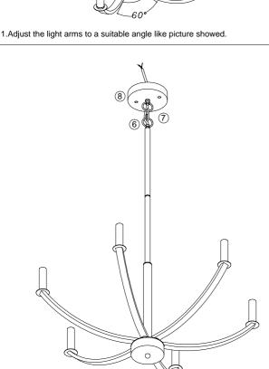
3.Connect the ring 6 with canopy 8 by carabiner hook screw connection 7, let the wire go through the canopy 8.
