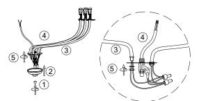
1.Install the arms 3 to the light fixture 4 with lock nut & teeth lock washer 5, install the bottom cover  $\ensuremath{@}$  to the fixture  $\ensuremath{@}$  with end cap  $\ensuremath{@}$ (Be carefully when install the arms to avoid damaged the wires!!!)
