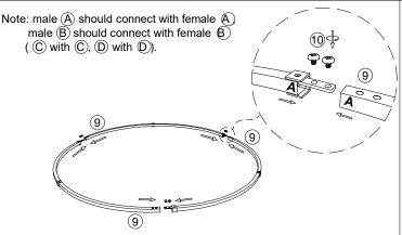
3. Assembled the split parts 9 to a completely ring fixture like picture showed, pushed the split parts together and fix with bolt screw (1).
