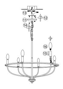
6.Install the bracket to the ceiling junction box with screw ①.
