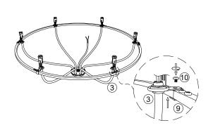
4.Put the ring 9 to the hook of the arms ③, adjust the position of the hole and fixed the ring  $\ensuremath{\mathfrak{D}}$  with screw  $\ensuremath{\mathfrak{D}}$ .
